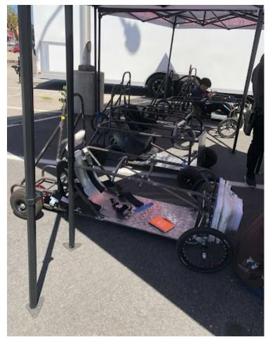
The chassis of Spectre consists of a hollow steel frame and a teardrop-shaped fiberglass body. The Scott DC motor is placed at the rear of the car, and powered by two ExpertPower batteries located behind the driver. The motor is mounted at the back of the vehicle on a newly machined aluminum plate. The vehicle has two Maxxis 16x1.95 inch wheels in the front and a Maxxis 20x1.95 tire for the rear wheel. Steering for the vehicle is done through hollow steel lever tubes.
